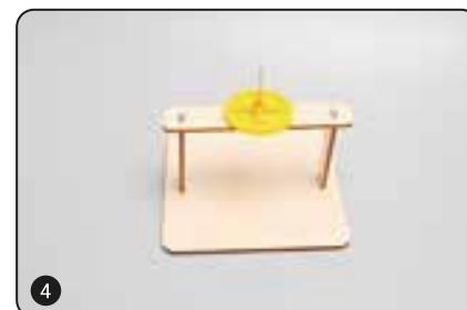
**EN** First install the support plate on the short support plate with 7mm screws, and then install the 3cm long iron shaft on the middle round hole of the pulley.(Do not use excessive force to install the iron shaft, it is easy to crush the support rod).
